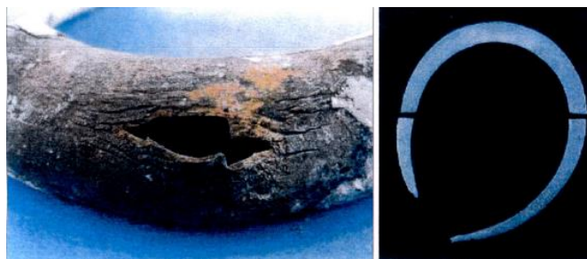
Figure 1: Leakage due to creep caused by oxide accumulation on the tube inner surface
